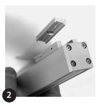
Move sliders on MOMO Sauna base to match plate spacing. Lock slider in position (grub screw/hex key).
